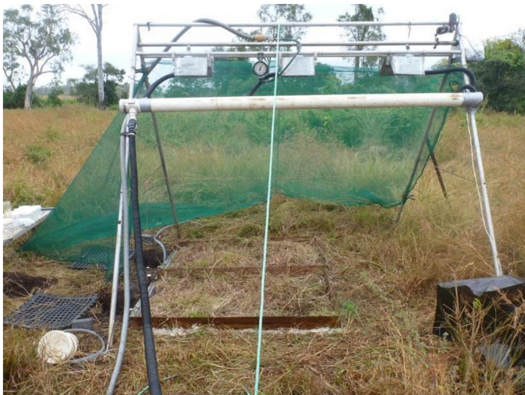
Figure 3.1: Rainfall simulation being undertaken. Water is applied via three nozzles each contained within a metal shroud (silver boxes toward the top of the picture). Two plots can be seen under the simulator. The nozzles oscillate across the plots (front to back in this picture) with runoff exiting through the plot end installed on the downslope end of the plot (left of picture).
